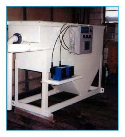
untreated wastewater. The layer of oil in most oil/water separators is typically pumped out on a regular basis and sent for recycling (see <u>Chapter 7, Hazardous and Recycled Waste</u>).
